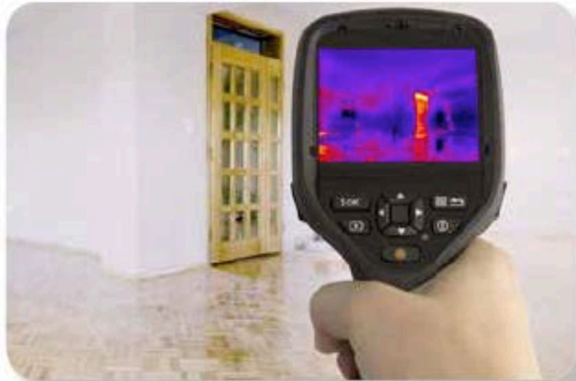
Infrared camera identifying air leakage.
