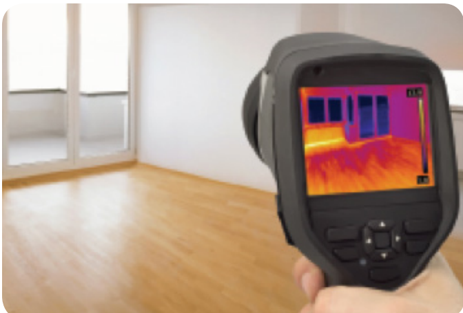
Infrared camera identifying air leakage.
