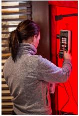
A blower door test was performed at the end of construction to test the air infiltration through the building envelope. The building performed outstanding.
